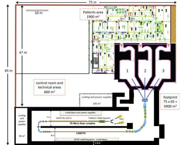
Figure 16: Preliminary layout of the all-linac carbon ion facility based on high efficiency design.
