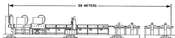
Figure 2: Schematic layout of the model PL-250 proton therapy linac designed by R. Hamm, K. Crandall and J. Potter [6].
