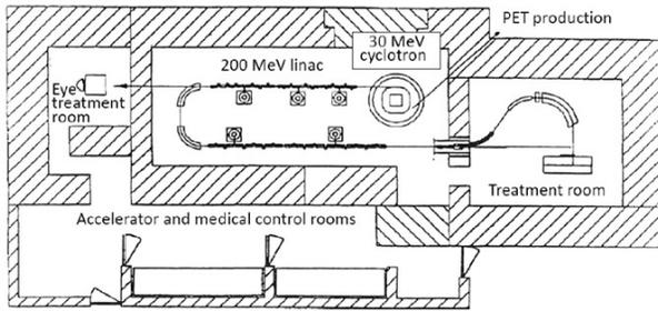
Figure 3: Schematic layout of the first “cyclinac” approach to proton therapy proposed in 1994 by one of the authors [7].
