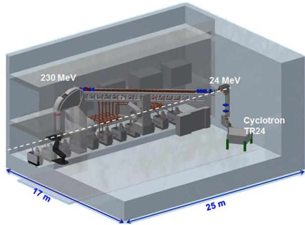
Figure 12: First design of the 11 m long TULIP; the injector is a 24 MeV commercial cyclotron.
