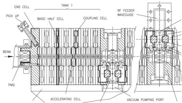
Figure 4: In this drawing of LIBO an accelerating cell and a coupling cell are highlighted in black.
