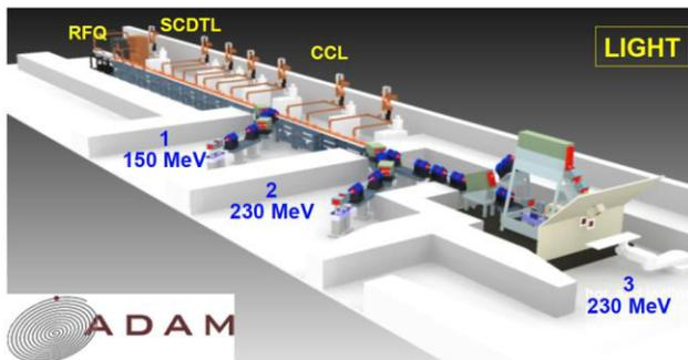
Figure 7: Layout of LIGHT, which is composed of three linear accelerators: RFQ (up to 5 MeV), SCDTL (up to 35 MeV) and CCL up to 230 MeV.
