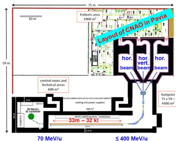
Figure 14: Preliminary layout of the linac based carbon ion facility based on high efficiency design.
