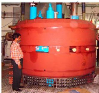
Figure 15: The Indian Variable Energy Cyclotron weighs about 100 tons [23].
