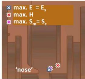
Figure 10: In a hadron linac the maximum surface electric field is close to the point of the nose.
