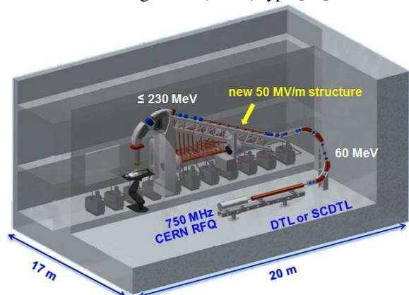
Figure 13: TULIP 2, based on a BTW linac, is 6 m long.
