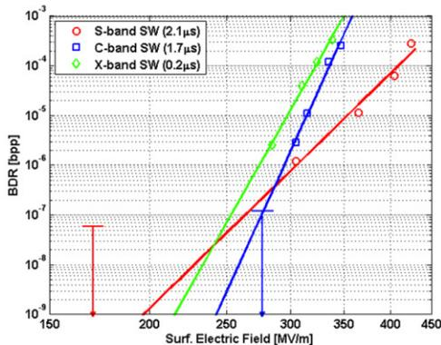
Figure 11: Comparison of results of BDR measurements performed at different frequencies [18].
