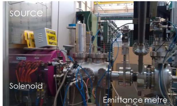
Figure 2: Set-up for emittance measurements at 45 keV.
