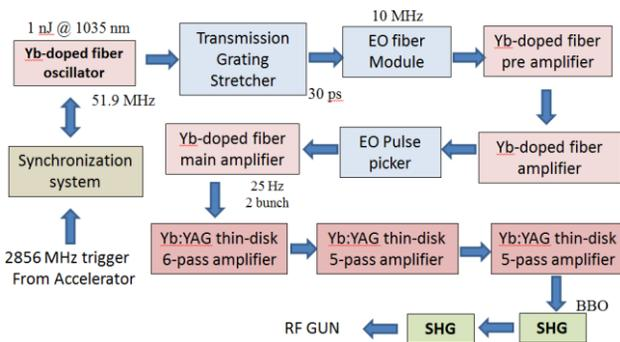
Figure 12: Layout of laser system.
