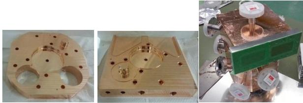
Figure 7: Photo of manufactured cells after brazing.
