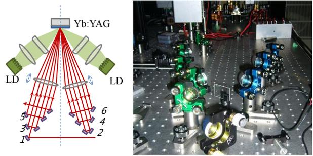
Figure 13: Thin-disk multi-pass amplifier.
