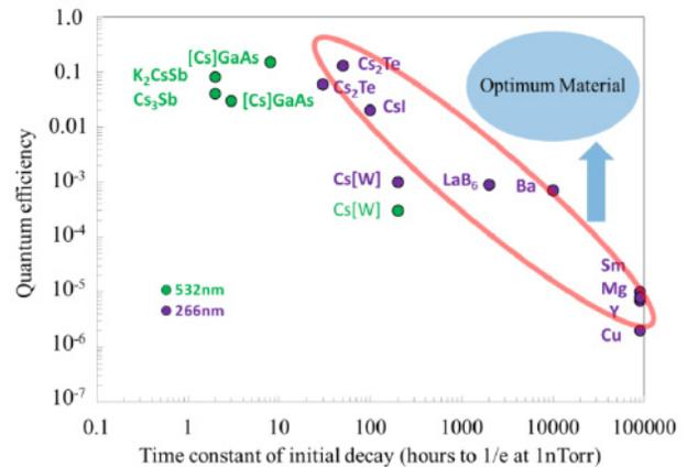
Figure 9: Quantum efficiency vs cathode lifetime.
