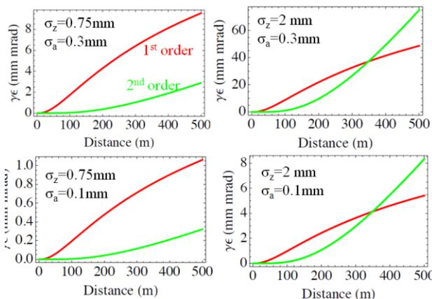
Figure 16: Analytical emittance growth due to misalignment.
