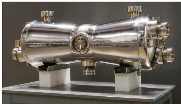
Figure 1: The 162.5 MHz,  $\beta = 0.11$ , niobium half-wave resonator enclosed in an integral stainless-steel helium vessel. The cavity is 125 cm end-to-end.
