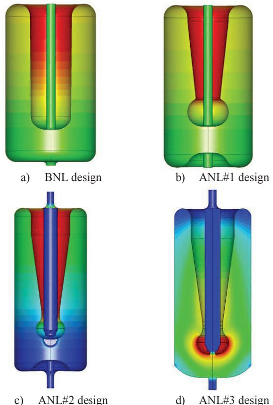
Figure 1: Cavity electromagnetic design progress (electromagnetic field distribution)
