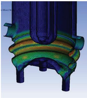
Figure 5: Von Mises stresses distribution for bellows tuner
