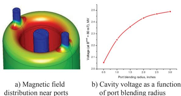
Figure 2: Local magnetic field on the port connection to the cavity
