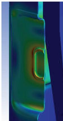
Figure 6: Von Mises stresses distribution for magnetic region tuner
