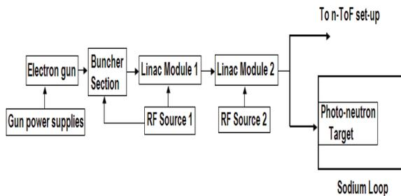
Figure 2: Schematic of 30 MeV RF Linac system for neutron generation
