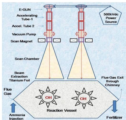
Figure 6: Conceptual design of EBFGT system
