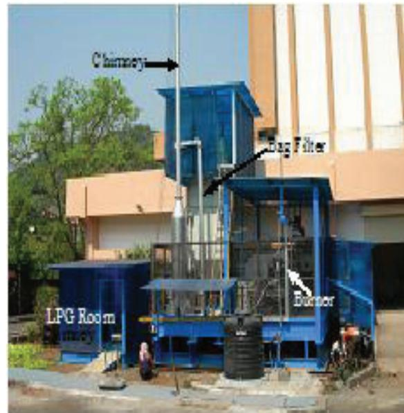
Figure 4: View of simulated plant for flue gas treatment
