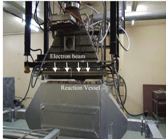
Figure 3: View of Reaction vessel below the electron beam
