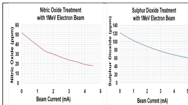
Figure 5: Reduction in SO<sub>x</sub>/NO<sub>x</sub> with electron beam
