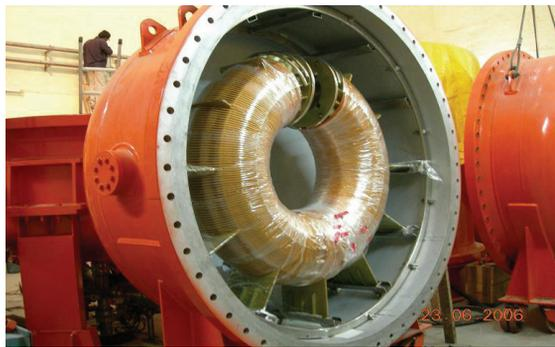
Figure 3: Transformer installed inside pressure vessel
