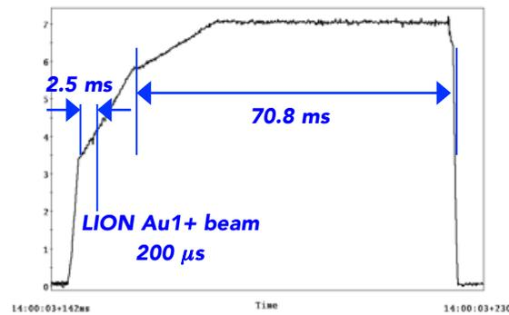
Figure 4: Injection timing using the LION
