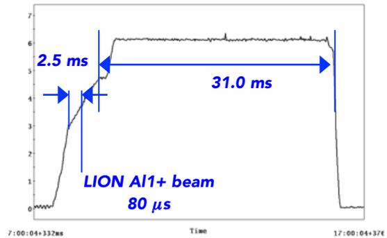
Figure 6: Injection timing for  $Al^{8+}$
