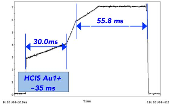
Figure 3: Injection timing using the HCIS
