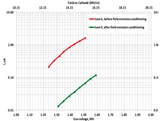
Figure 8: Dark current measured before and after conditioning.
