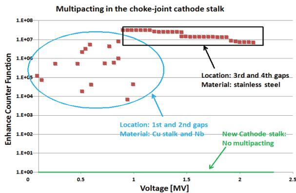
Figure 4: Multipacting simulation results in the quarter-wavelength choke joint.
