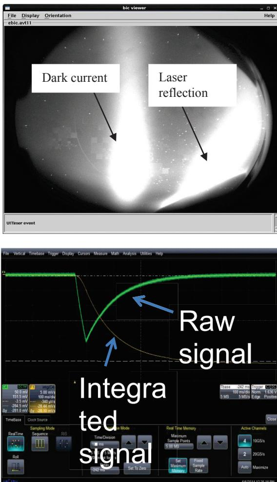
Figure 7: Dark current image on YAG screen (above) and dark current measured by faraday cup (bottom).
