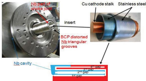
Figure 2: Quarter-wavelength cathode stalk insertion.
