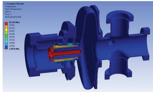
Figure 5: Thermal analysis of the new cathode stalk.
