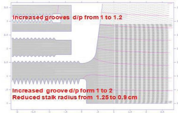
Figure 3: New design of a multipacting-free cathode stalk.
