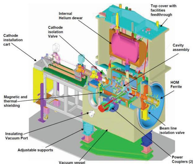
Figure 1: SRF gun cryomodule.
