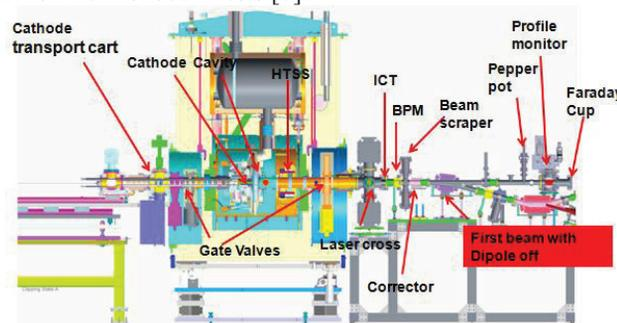
Figure 6: First beam commissioning configuration.
