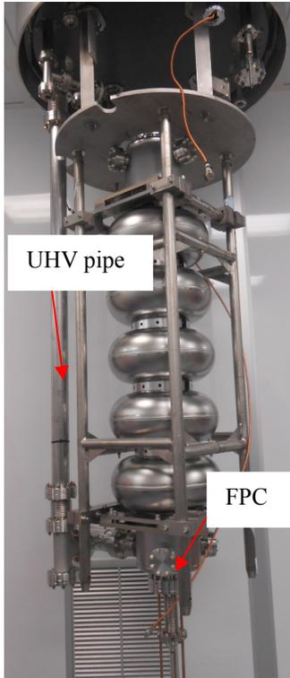
Figure 2: Setup of the BNL3 cavity vertical test.
