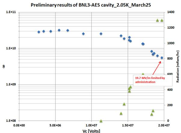
Figure 5: Vertical test results of the BNL3-AES cavity.
