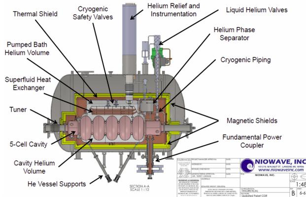
Figure 6: The BNL3-AES cavity in a cryomodule under fabrication at Niowave.
