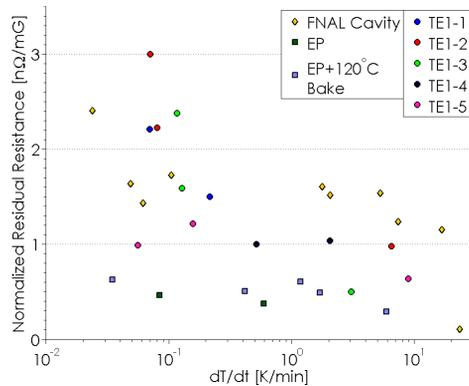
Figure 5: Residual resistance normalized to the external field as a function of cool down rate through  $T_c$  for the eight cavities.
