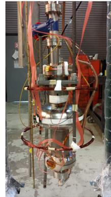
Figure 1: The experimental setup showing cavity, coil for applying magnetic field, fluxgate magnetometers, and temperature sensors.
