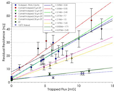
Figure 2: Residual resistance as a function of trapped flux. The amount of flux trapped in the cavity walls depends on both applied field and cool down rate (gradient) [3].
