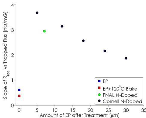
Figure 3: Slope of linear fit from Fig. 2 as a function of final EP after treatment. The FNAL cavity was given a nitrogen doping at a lower pressure than the Cornell cavities, giving it a lower N-doping level and thus a lower susceptibility to trapped flux for the same final EP.
