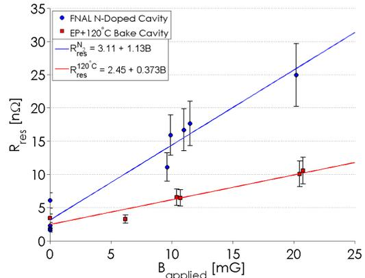
Figure 4: Residual resistance vs applied magnetic field under fast (>1 K/min) cool down conditions.
