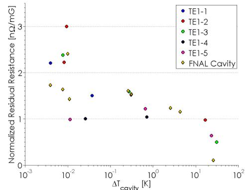
Figure 6: Residual resistance normalized to the external field as a function of temperature gradient across the cavity when it transitions from normal to superconducting for the eight cavities.
