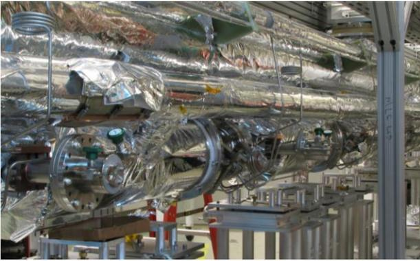
Figure 7: Cold couplers mounted on the linac cavities during cold mass assembling of main linac cryomodule.
