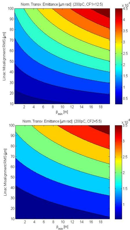
Figure 3. Normalized RMS projected emittance at the entrance of BC2 (top) and linac exit (bottom), as function of the linac-to-beam RMS misalignment and the horizontal betatron function in the BC1 (top) and BC2. The plot on the top assumes an initial emittance of 0.15 μm, the plot on the bottom 0.5μm.
