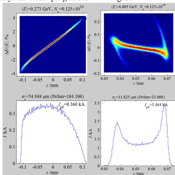
Figure 2. Longitudinal phase space (top) and current profile (bottom) at the exit of BC1 (left) and linac end. The RMS energy spread is, respectively, 1.8% and 0.05%.
