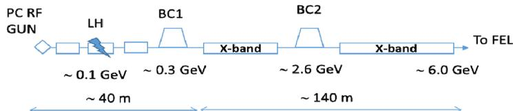
Figure 1: 6 GeV linac layout.
