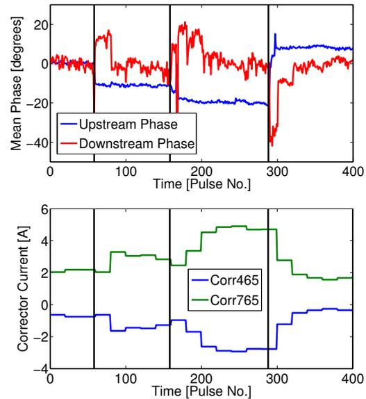
Figure 5: Mean phase (top) and corrector settings (bottom) during the slow correction run. Vertical lines mark the times that the phase was shifted using the stretching chicane.
