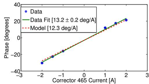
Figure 4: Dependence of phase measured in the downstream monitor on the corrector currents.
