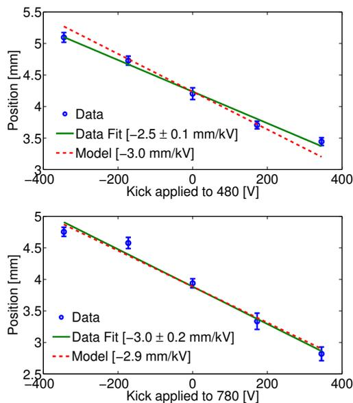
Figure 6: Response to the first (top) and second (bottom) kicker in the first BPM after the chicane.
