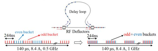
Figure 3: The bunch combination in the delay loop [1].
