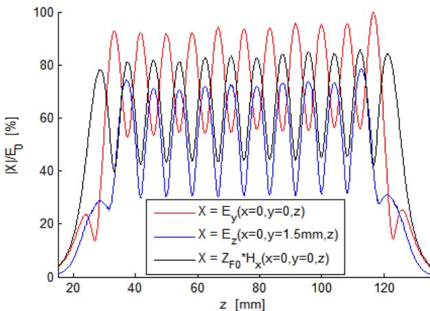
Figure 3: Comparison of different field components  $E_y$ ,  $E_z$  and  $Z_{F0}H_x$  along the cavity in the vicinity of the axis.  $E_z$  rises linearly with an offset in  $y$ -direction.
