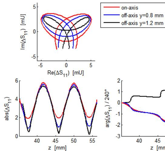
Figure 4: Change of input reflection  $\Delta S_{11}$  for a bead running on axis ( $x=0, y=0$ ) and off-axis ( $x=0, y=0.8 / 1.2$  mm) through two regular cells. Top:  $\Delta S_{11}$  in the complex plane, bottom left: magnitude of  $\Delta S_{11}$  and bottom right: normalised phase of  $\Delta S_{11}$  along the longitudinal direction.
