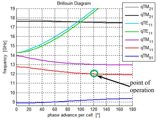
Figure 2: Mode spectrum of the first seven modes. The operating quasi-TM<sub>11</sub>-mode (red) is well separated in frequency from the fundamental mode and the higher order modes, including the  $x$ -polarised quasi-TM<sub>11</sub>-mode (purple).
