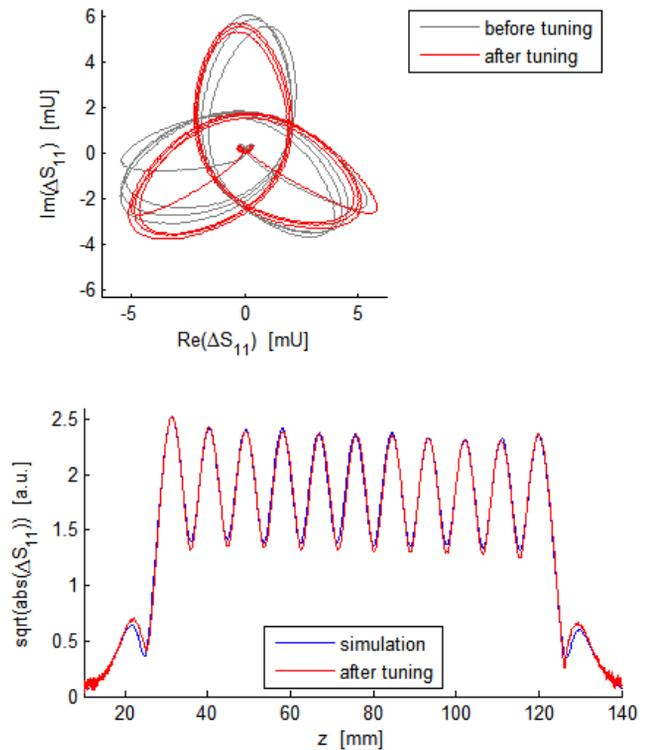
Figure 6: Bead-pull measurement results before (grey) and after (red) tuning compared to simulations (blue).
