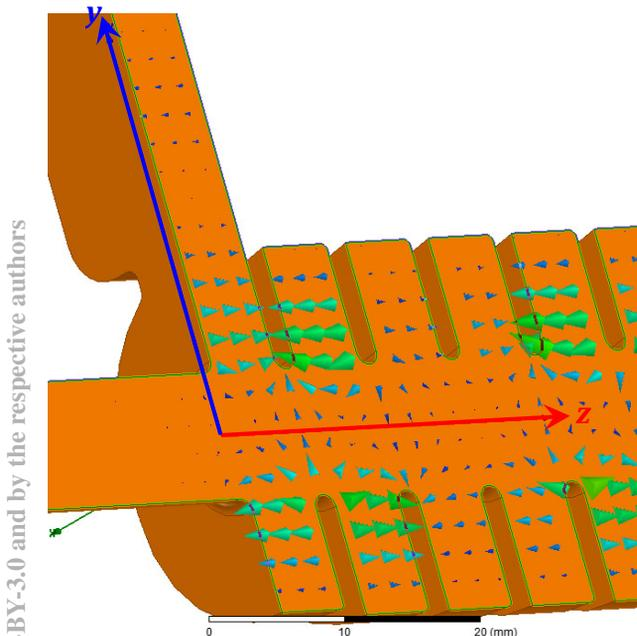
Figure 1: Electric field distribution of the deflecting quasi-TM<sub>11</sub>-mode in a cross section of the crab cavity. The power is fed into the structure via the input coupler (top left). The following coordinate system is used:  $z$  is the beam axis and  $y$  is the direction of desired deflection.
