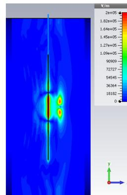
Figure 3: Calculated bunch electric field for conditions expected at LBM4 location.
