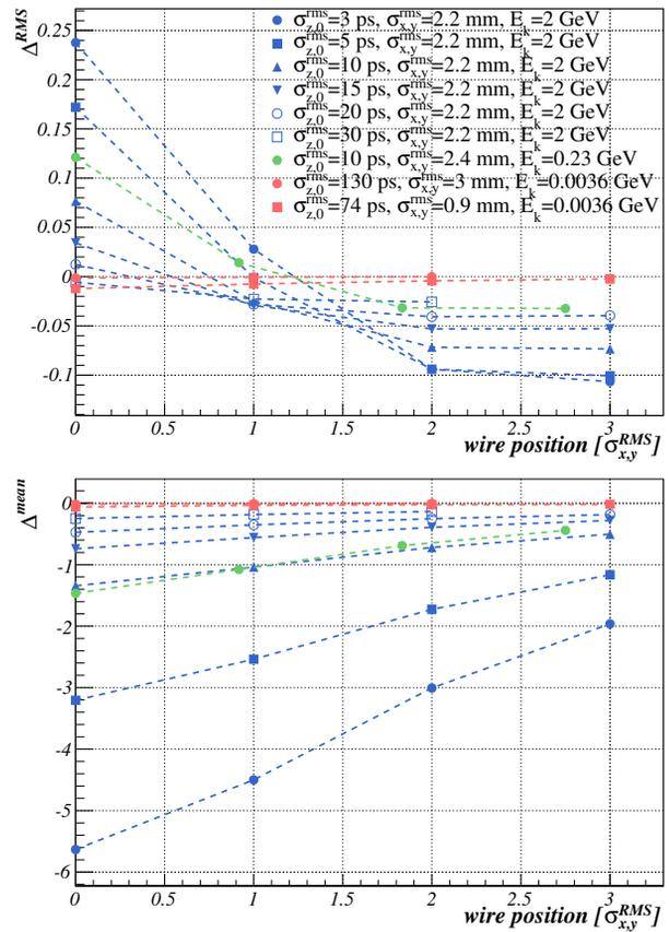
Figure 5: Expected normalized difference in RMS (top) and mean (bottom) of the SE time distributions at the beam pipe boundary as a function of wire position in units of one-sided RMS beam transverse size  $\sigma_{x,y}^{\text{RMS}}$ .
