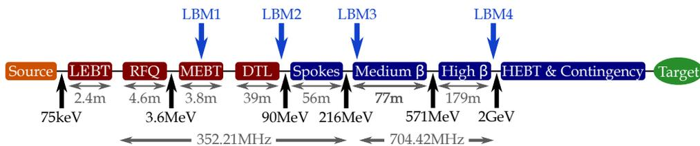
Figure 1: ESS linac and LBM layout.
