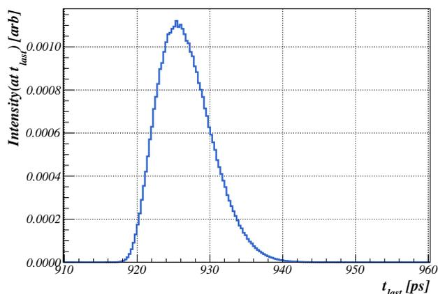
Figure 4: Time distribution of the SEs at the beam pipe boundary for conditions expected at LBM4 location.
