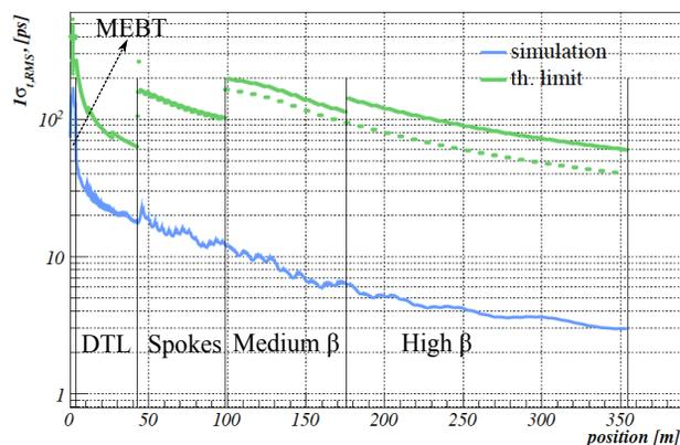
Figure 2: Expected one-sided RMS bunch lengths at the ESS linac (blue) and intrinsic limit on the one-side RMS length due to the spatial spread of charge field (green).
