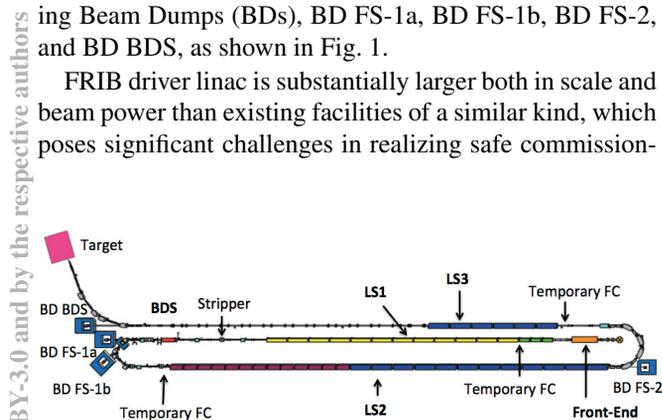
Figure 1: Schematic layout for FRIB driver linac.
