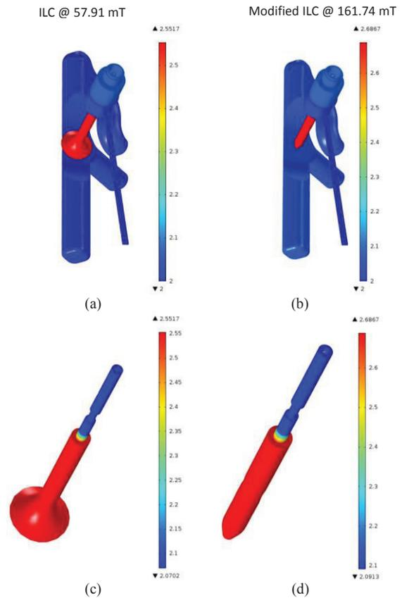
Figure 8: Thermal profile of both; the conventional ILC antenna and the modified one. (a) ILC antenna assembly. (b) Modified ILC antenna assembly. (c) ILC antenna. (d) Modified ILC antenna.
