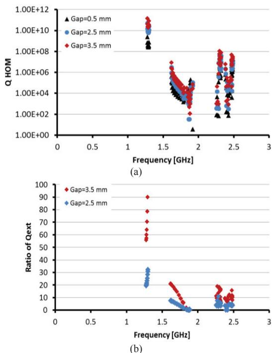
Figure 3: Effect of trimming the HOM antenna. (a)  $Q_{ext}$ . (b) Ratio of  $Q_{ext}$ .
