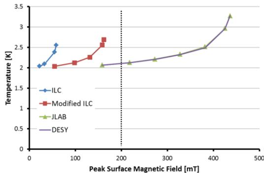
Figure 7: Antenna tip temperature versus peak magnetic field for the proposed modified antenna compared to ILC, JLAB and DESY designs.
