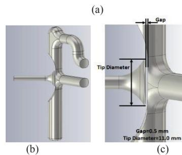
Figure 2: The geometry of the HOM coupler and antenna for the ILC cavity (a) Transparent front view of the cavity showing the HOM couplers (b) HOM antenna and f-part. (c) Dimension of HOM antenna.
