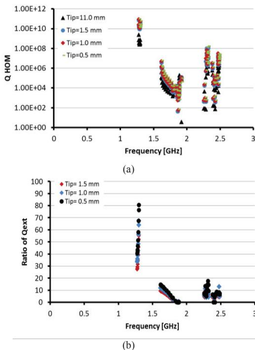
Figure 5: Effect of reducing the size of the HOM antenna. (a)  $Q_{ext}$ . (b) Ratio of  $Q_{ext}$ .
