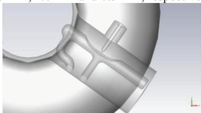
Figure 4: Reducing tip size of the HOM antenna.
