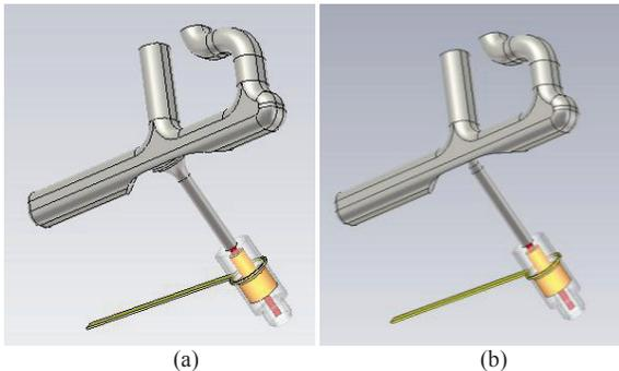
Figure 6: HOM antenna assembly, Niobium antenna and f-parts, Alumina ceramic, Stainless Steel pin, Stainless Steel sleeve, and the Copper cooling lead. (a) ILC style. (b) Modified ILC style.
