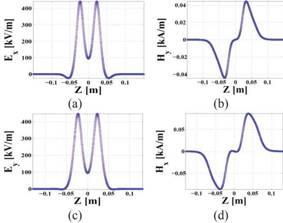
Figure 2: Transverse fields on axis for inner conductor displacement along X, (a) and (b), and Y (c) and (d).
