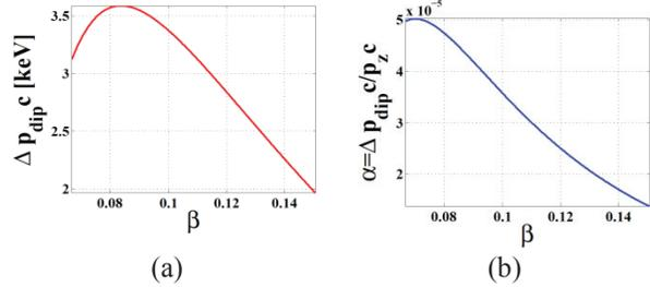
Figure 8: Dipole kick on axis (a) and  $\Delta p_{\perp}c/p_zc$  (b) as function of beta for trimmed HWR.
