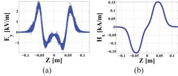
Figure 7: Electric (a) and magnetic (b) transverse fields on axis, due to asymmetric trim of the HWR.
