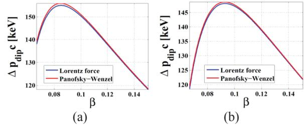
Figure 3: Transverse kick vs beta, (a) X and (b) Y electrode displacement.
