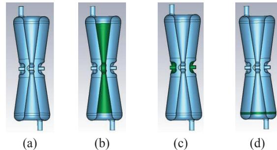
Figure 1: HWR geometry Y-Z section (a), inner electrode highlighted (b), beam tubes highlight (c), area of asymmetric trimming shown in green (d).
