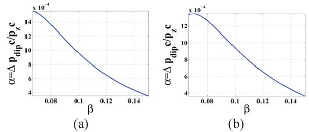
Figure 4:  $\alpha$  vs particle beta for HWR inner electrode displacement in X (a) and Y (b) axis.
