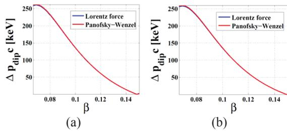
Figure 6:  $\Delta p_{\perp}c$  vs  $\beta$ , Lorentz's force and Panofsky-Wenzel's calculation for beam pipes displacement X (a) and Y (b).
