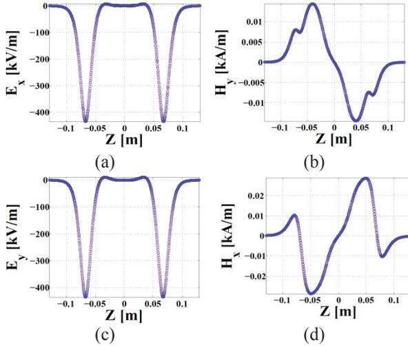
Figure 5: Transverse fields on axis due to beam pipe displacements (a) and (b) 1 mm X, (c) and (d) 1 mm Y.
