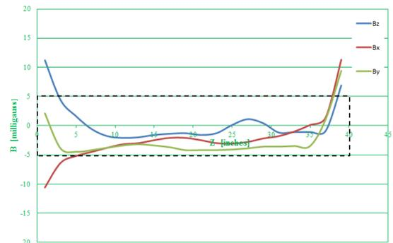
Figure 1: Room temperature magnetic field profile along the length of an ILC helium vessel/magnetic shield installed in HTS with cancellation coils turned on. The z-direction is along the cavity axis (north-south in HTS), the y-direction is vertical, and the x-direction is transverse. The dotted outline represents the LCLS-II target and the extent of the helium vessel/shielding.
