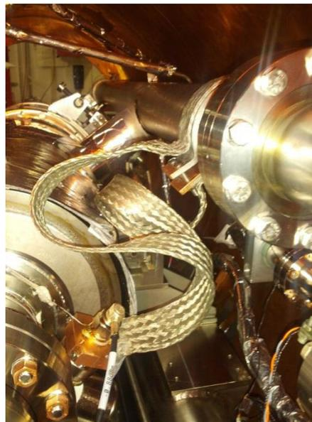
Figure 4: A DESY HOM feedthrough connected via copper braid to the two-phase helium header.
