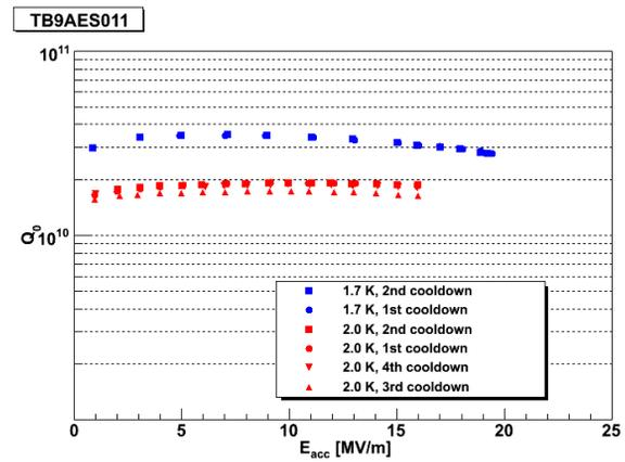
Figure 5:  $Q_0$  vs.  $E_{acc}$  curves for TB9AES011 after the cooldowns described in Tab. 1.
