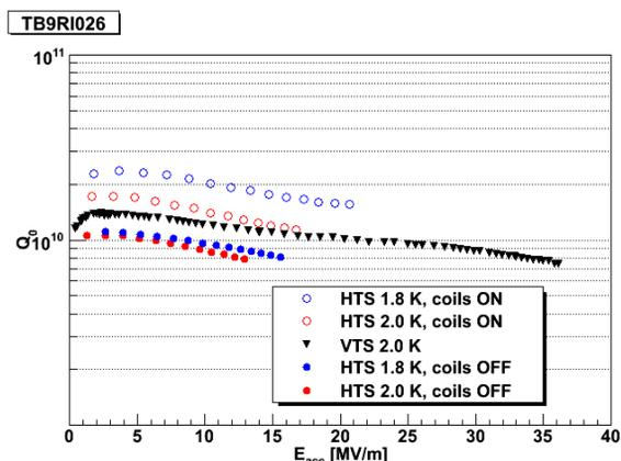
Figure 2:  $Q_0$  vs.  $E_{\text{acc}}$  curves for HTS and VTS. "Coils ON/OFF" refers to the state of the magnetic field cancellation coils when the cavity was cooled through the critical temperature  $T_c$ .
