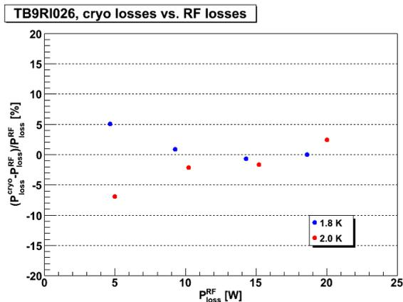
Figure 3: Percent difference between RF measurements of cavity losses  $P_{\text{loss}}$  and cryo measurements of same, at various values for  $P_{\text{loss}}$ .
