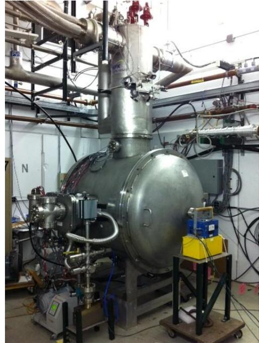
Figure 1: The Spoke Test Cryostat with upgraded feed can.
