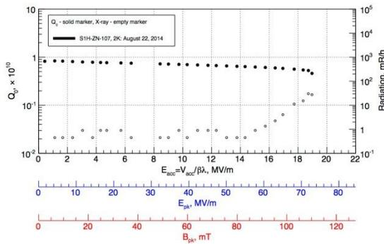
Figure 6:  $Q_0$  vs.  $E_{acc}$  curve and X-rays for S1H-NR-107.
