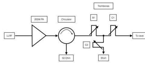
Figure 4: Phase shifter matching network implemented to minimize and measure circulator reflection effects. "C1" is the phase shifter varied to produce Fig. 3.
