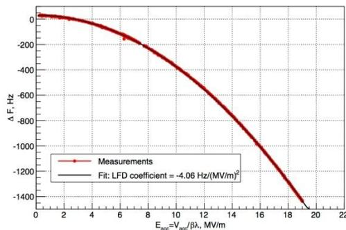
Figure 7: Detuning of S1H-NR-107 from Lorentz forces at various gradients. The black curve is a second-degree polynomial fit to the data (red points).
