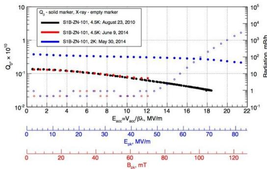
Figure 2:  $Q_0$  vs  $E_{acc}$  curves taken at 2 K (blue) and 4.5 K (red) for cavity S1Z-NR-101 at the upgraded STC. The black points are the 4.5 K data for the cavity's STC test prior to the upgrade. X-ray flux is also shown (open circles).
