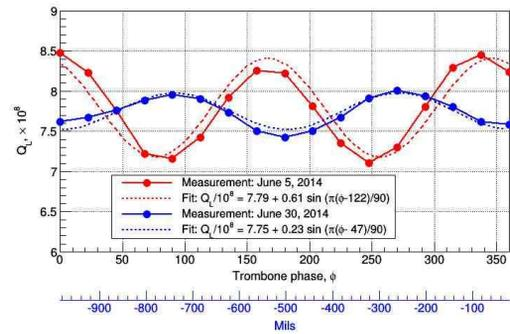
Figure 3: Variation in  $Q_L$  with phase delay. The data shown in blue and red correspond to with and without the matching network of Fig. 4, respectively.
