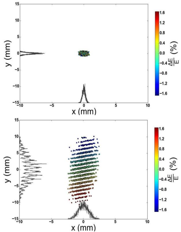
Figure 5: The transverse profile of the electron beam with the slits inside the beamline. The upper figure is the image on the transverse profile monitor YAG/OTR when the skew quadrupole is turned off and the lower figure when the skew quadrupole is turned on. The skew quad in effect functions like an RF deflector albeit imperfect
