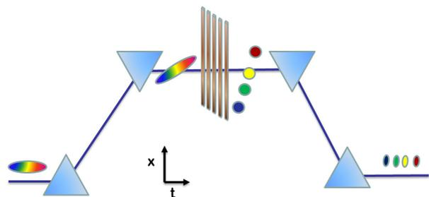
Figure 1: Schematic of the ASTA bunch compressor with the Z-Slicer.
