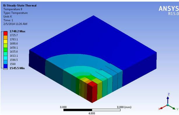
Figure 4: Steady state thermal analysis of the quarter of the slit-maks assuming the beam is hitting the center of the slits.
