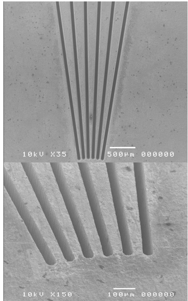
Figure 2: SEM images of the multi-V slits (top) showing the change of the distance between the slits as a function of transverse position. The bottom SEM image is on the exit side of the slits showing the topography.
