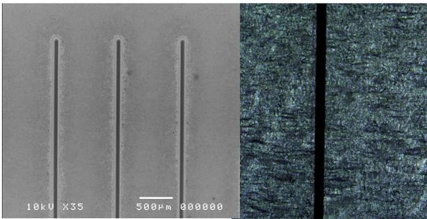
Figure 3: The SEM image of a standard multi-slit (left) with the Laser Scanned Microscope image (right). The LSM measurement yields  $47.4 \mu\text{m}$  as the width of the slits
