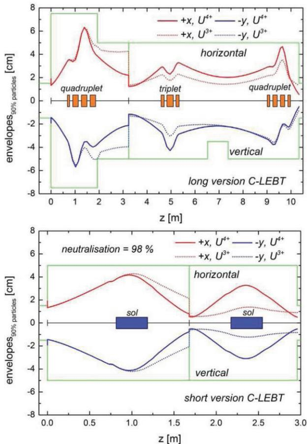
Figure 3: The preferred LEBT solution (top) in comparison with an alternative concept for the LEBT comprising two solenoids [4].
