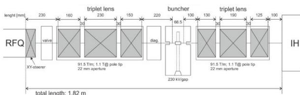
Figure 4: An alternative concept for the MEBT instead of the existing doublet-superslens combination [6].
