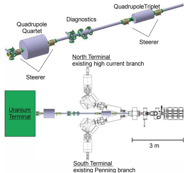
Figure 2: The existing HSI-LEBT branches together with the planned straightforward injection.
