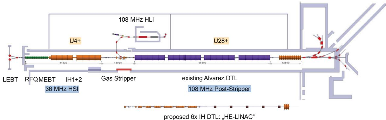
Figure 6: The existing GSI linear accelerator UNILAC with an Alvarez DTL behind the gas stripper. The Alvarez is proposed to be substituted by an IH DTL, the so-called HE-Linac [8].
