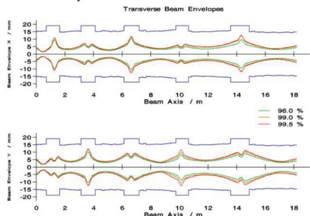
Figure 5: Transverse envelopes through the HE-Linac.
