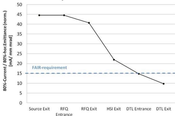
Figure 1: Beam quality along the UNILAC including future upgrade options like the Compact LEBT already with the existing Alvarez DTL [2].
