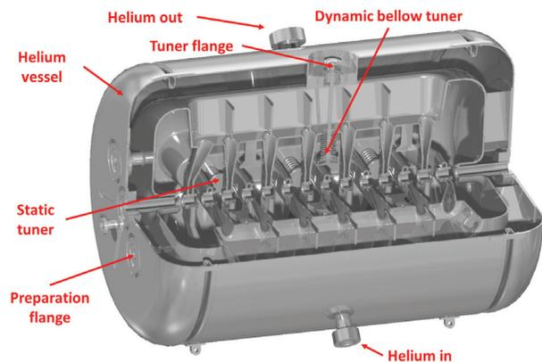
Figure 2: 3D-model of the sc 217 MHz CH cavity.
