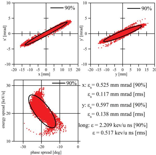
Figure 7: Output particle distribution of the IH-DTL with optimized MEBT.
