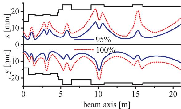
Figure 6: Transversal beam envelopes of the IH-DTL using the input from the proposed MEBT design. Apertures are plotted in black.
