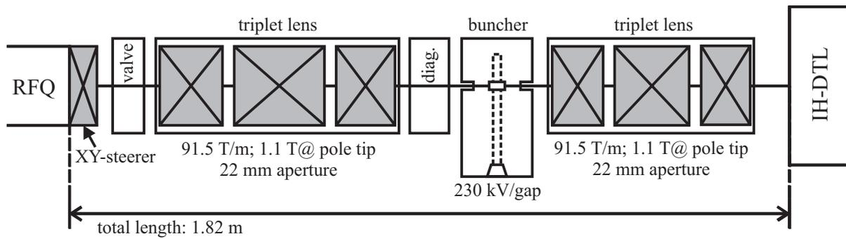
Figure 3: Layout of the proposed MEBT section showing all components including the valve, XY-steerer and diagnostics box from the current MEBT section.
