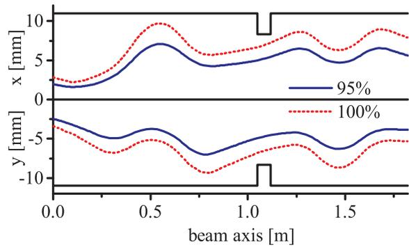
Figure 5: Transversal beam envelopes of the proposed MEBT design. Apertures are plotted in black.
