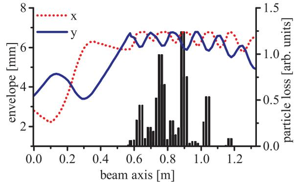
Figure 1: Loss profile of the current MEBT superlens for 20.75 mA  $U^{4+}$ . Plotted beam envelopes are 100 %, the superlens aperture is 6.8 mm.
