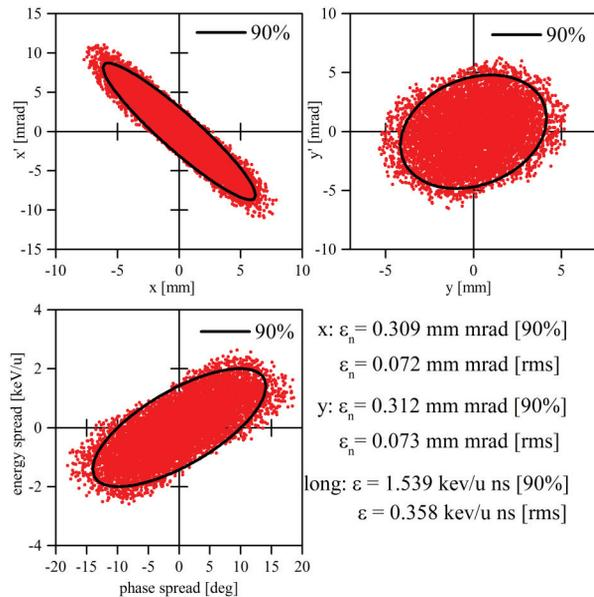
Figure 4: Output particle distribution of the proposed MEBT section.
