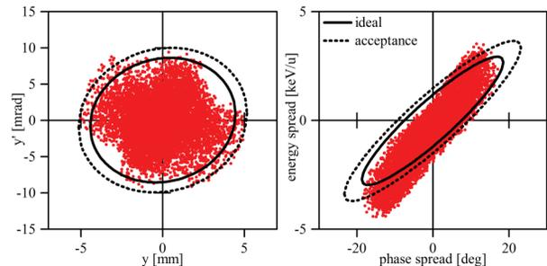
Figure 2: Output distributions of the superlens MEBT with IH-DTL acceptance ellipses.
