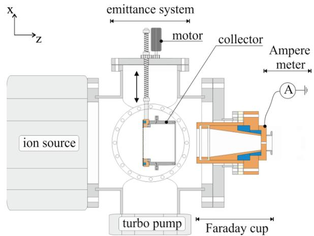
Figure 2: Experimental setup [2].
