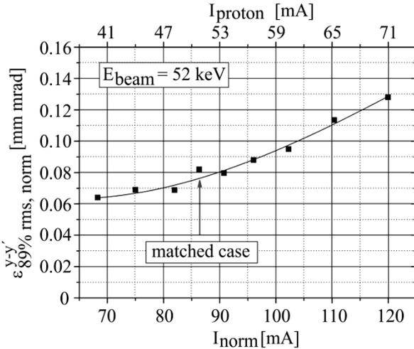
Figure 6: Measured 89% rms emittance depending on normalized beam current.
