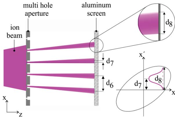
Figure 3: Pepper pot measurement principle.
