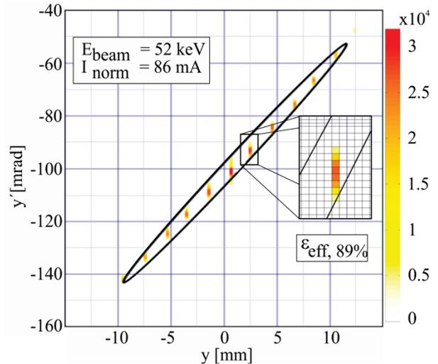
Figure 8: 89%  $y-y'$  rms emittance (52 keV@ $I_{norm}=86$  mA).
