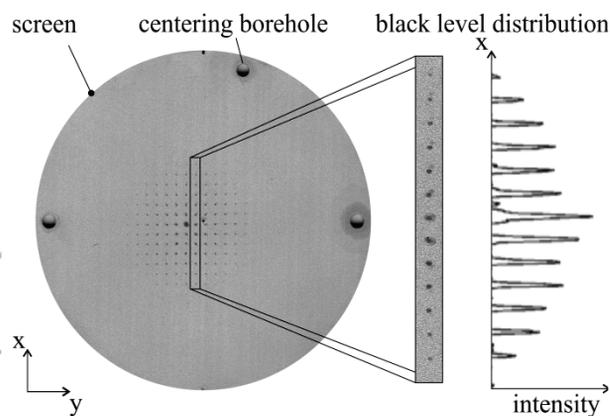
Figure 4: Aluminum screen with carbon footprints.
