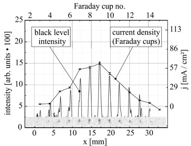
Figure 5: Footprints and current density distribution comparison.
