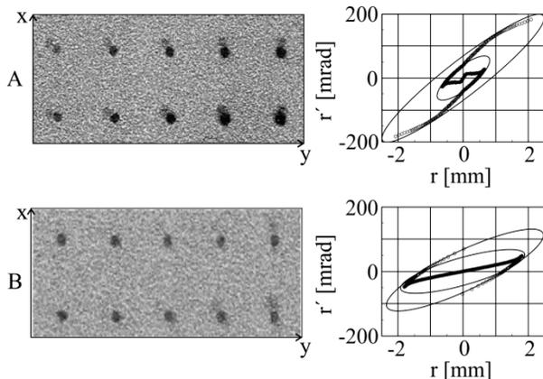
Figure 7: Footprints and IGUN phase space distribution for low plasma density ( $I_{norm}=68$  mA, above) and high plasma density ( $I_{norm}=120$  mA, below).
