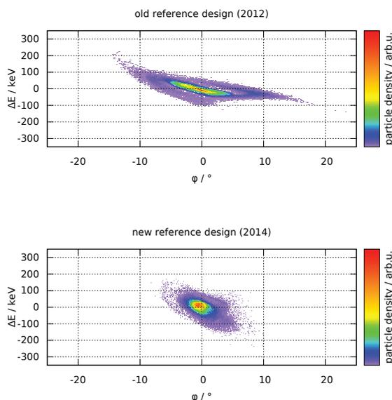
Figure 5: Longitudinal particle beam output distributions.
