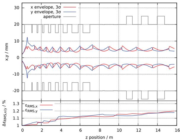
Figure 3: The periodic doublet lattice focuses the beam and ensures a small fill factor of the aperture. For an appropriate transversal focusing in the longer drift of the transition section the beam envelope widens to  $r_{beam,3\sigma} \approx 8.5$  mm.
