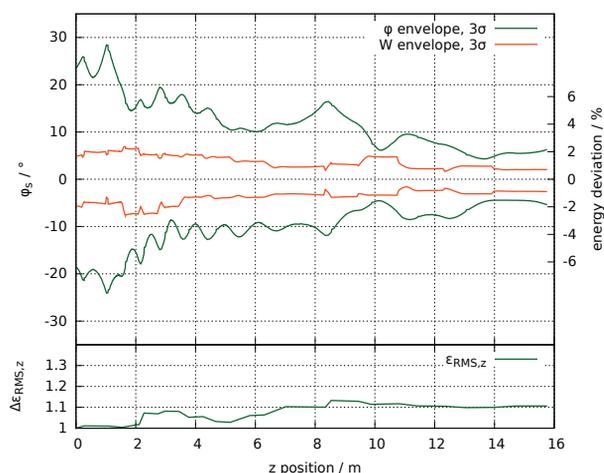
Figure 4: The longitudinal 3 $\sigma$  envelopes for the phase and energy spread of the beam (upper graph) with longitudinal RMS emittance growth rate (lower graph).
