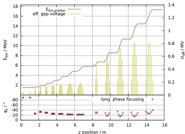
Figure 1: The kinetic proton energy after the 4-Rod-RFQ is  $W_p = 1.5$  MeV and increases up to  $W_p = 17.3$  MeV at the end of the CH section (upper graph, in red). The effective voltages of the gaps are plotted in yellow. In the lower graph the gap phase configuration of the RT constant phase structures and the SC constant  $\beta$  structures is visualized.
