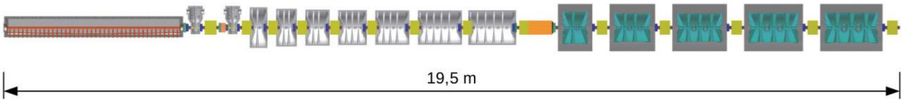
Figure 2: Cross sectional scheme of the components of the MYRRHA injector (without source and LEBT). The 4 m long 4-Rod-RFQ is followed by nine RT cavities (grey) and five SC cavities (blue). The quadrupol lenses (yellow), collimators and a lot of diagnostic devices are in between.
