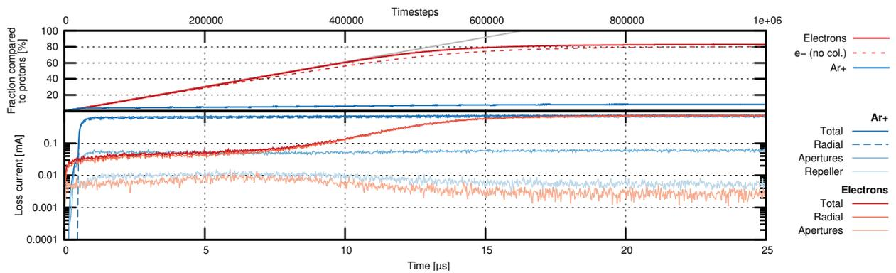
Figure 2: Particle population and losses during the built-up of space-charge compensation for the 50 cm drift system. The compensation degree is plotted for two different simulation runs: with and without electron induced ionization (dashed).
