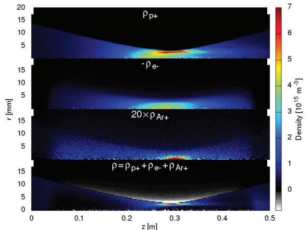
Figure 1: Proton, electron and residual gas ion particle densities in the simulation of the 50cm drift test system. The repeller electrodes at  $-1.5 \text{ kV}$  are visible at the front and the back of the system.
