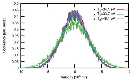
Figure 3: Electron spectrum at the center of the system in the steady-state.
