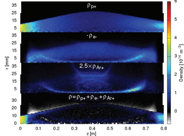
Figure 4: Particle densities for a system containing one solenoid 25 cm long at  $B_{max} = 378$  mT.
