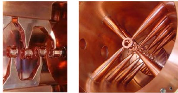
Fig. 1: IH - type (left) and CH - type (right) structure.
