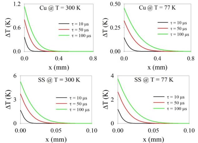
Fig. 7: Temperature profiles at the cavity surface at the end of specified pulse lengths.
