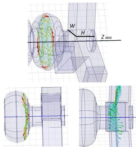
Figure 3: Magnetic field distribution for the TM<sub>211</sub> mode in the transition from last cell to damping region.
