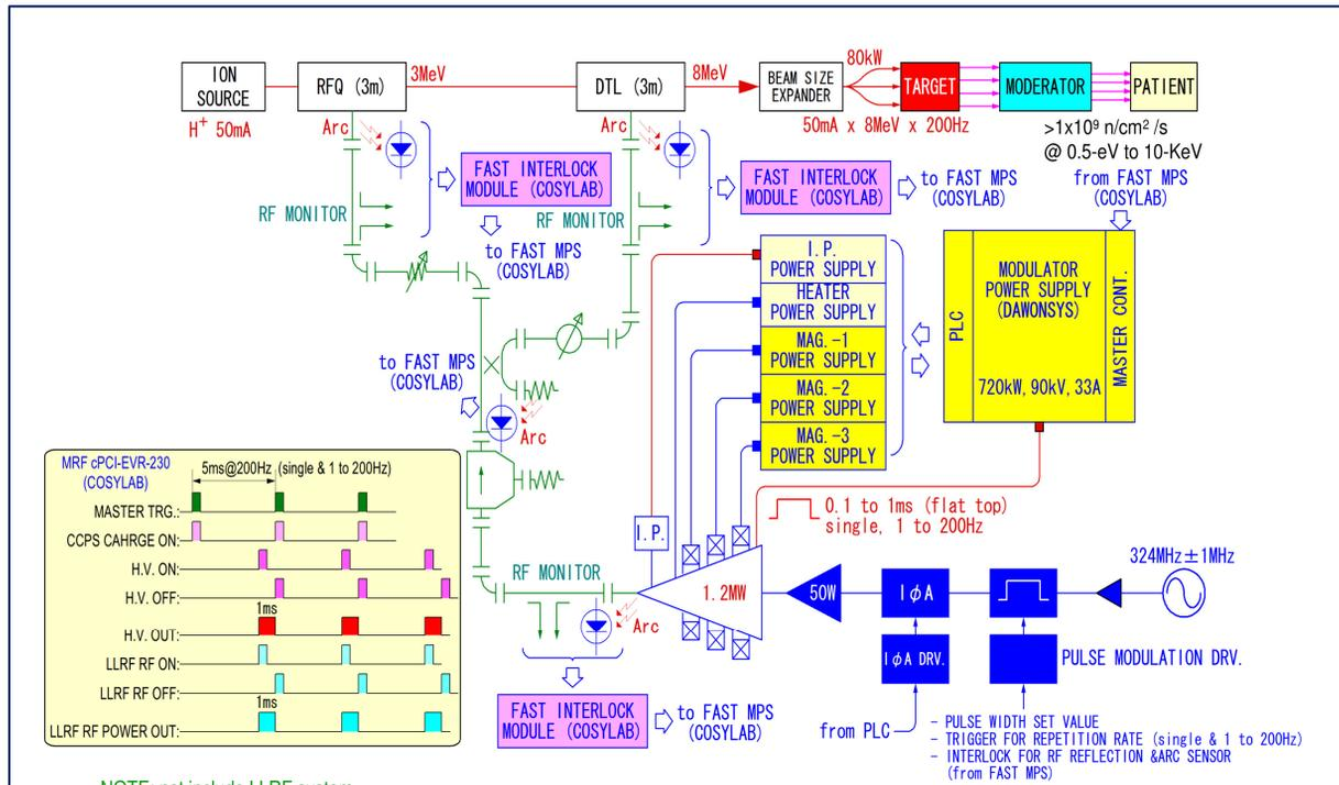
Figure 2: Block diagram of the RF system. The RF power from one klystron is split into two to feed the RFQ and DTL
