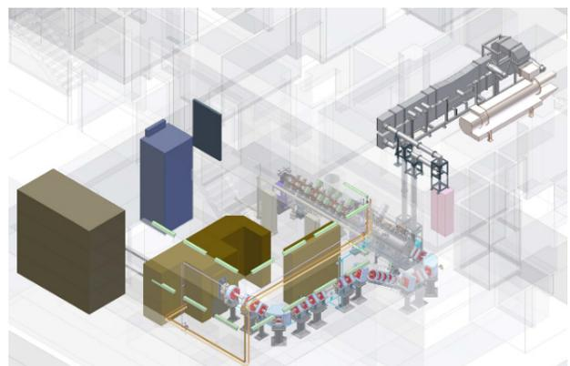
Figure 1: Layout of the i-BNCT, (left) Irradiation room, (middle) accelerator and (right) Klystron, modulator and LLRF, and magnet power supplies
