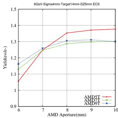
Figure 4: Yield as a function of AMD aperture for 5 Tesla (red), 7 Tesla (green), and 9 Tesla (blue) peak field. Aperture is given in radius.
