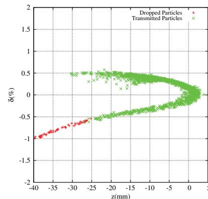
Figure 3: Particle distribution in longitudinal phase space at the end of the ECS. Green plot shows positron accepted by DR aperture and red plot shows dropped positron.
