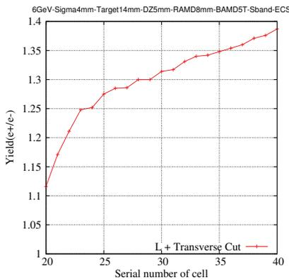
Figure 5: Yield as a function of cell number where L-band ends.
