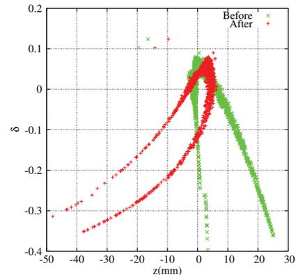
Figure 2: Particle distribution in longitudinal phase space at the end of the injector (green) and chicane (red).
