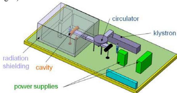
Figure 4: Layout to the test stand at GSI.
