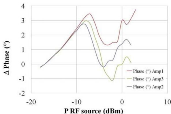
Figure 8: Phase variation vs input power.
