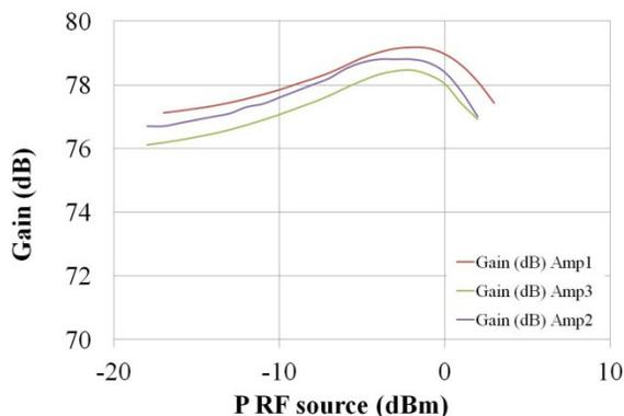
Figure 7: Gain vs input power.
