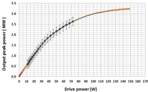
Figure 3: Power transfer curve @115kV 10 Hz 200 μs.
