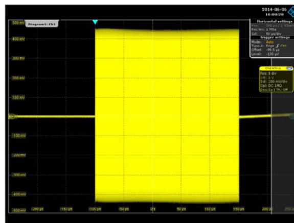
Figure 9: The RF pulse (50 μs/div) @ 45 kW.
