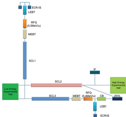
Figure 1: Layout of RAON superconducting linacs.
