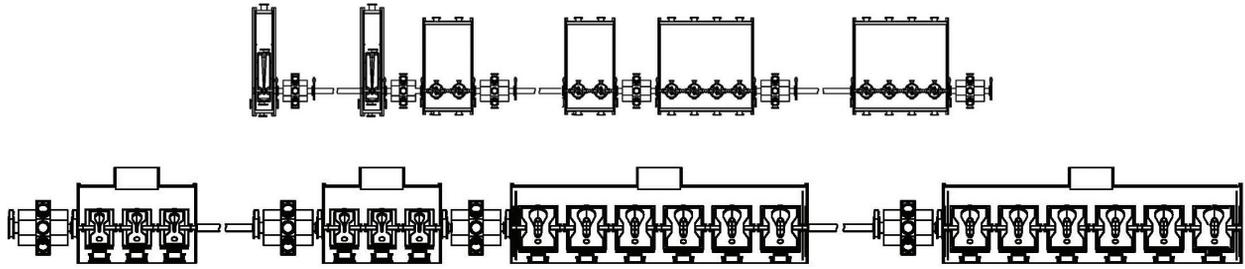
Figure 3: Layout of the superconducting linac: (top) low energy superconducting linac (SCL1 and SCL3), and (bottom) high energy superconducting linac (SCL2).
