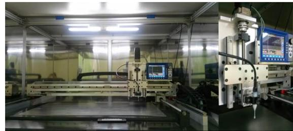
Figure 2: The ECT system for RAON's cavities.
