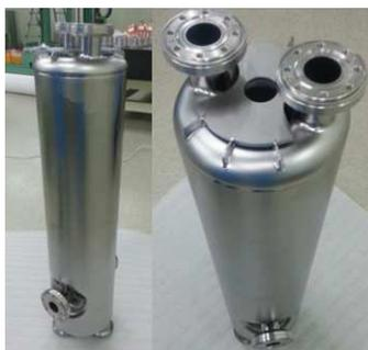
Figure 4: Prototype of quarter wave resonator.
