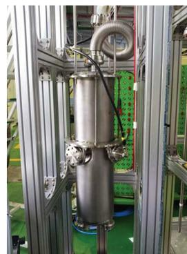
Figure 5: Prototype of half wave resonator.
