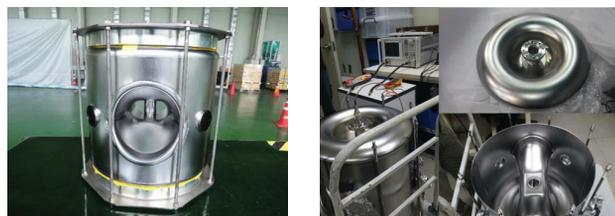
Figure 6: Prototyping of single spoke resonators: SSR1 (left) and SSR2 (right).
