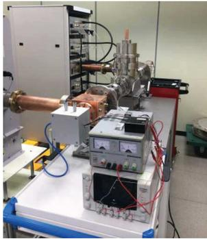
Figure 7: Prototyping of RF coupler.
