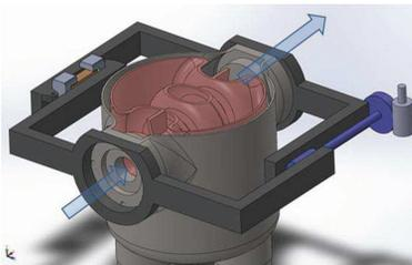
Figure 8: Layout of slow tuner for quarter wave resonator.
