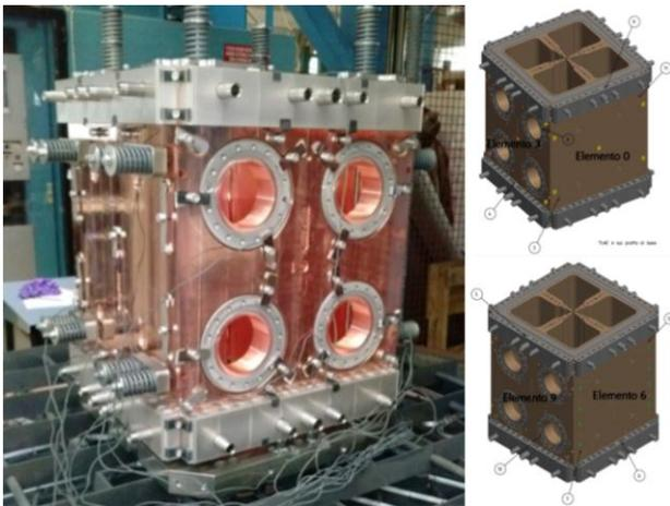
Figure 6: The M\_12 before the brazing cycle (left); the thermocouples position and number.
