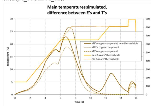
Figure 9: FEM simulated differential Temperature between components, considering an intermediate plateau (continuous line) or without (dotted line).
