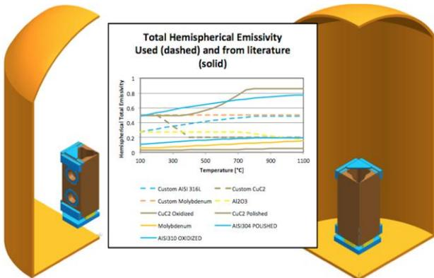
Figure 7: The Ansys FEM model of the Module in the brazing oven (sides); Table of the emissivity for the materials used at the brazing cycle temperatures.
