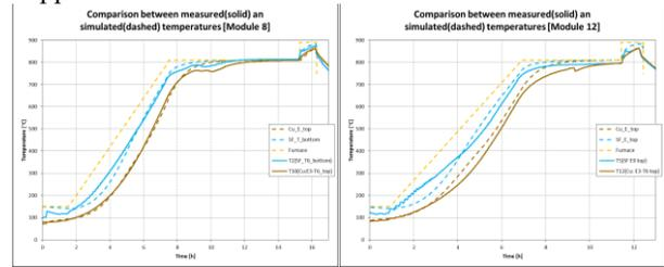
Figure 8: Comparison between the thermocouples data and the FEM simulation for low energy (left) and high energy Module geometry (right).
