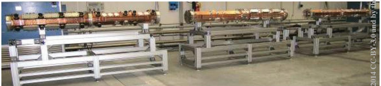
Figure 1: TRASCO RFQ modules.
