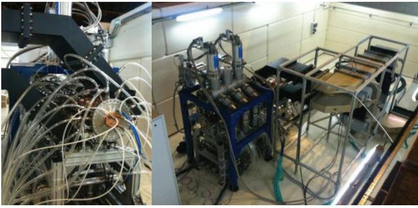
Figure 6: TRASCO RFQ during high power tests at CEA Saclay.
