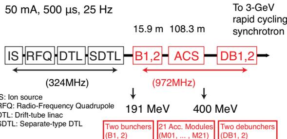
Figure 1: Diagram of the J-PARC linac accelerating structure in the 400-MeV beam operation.
