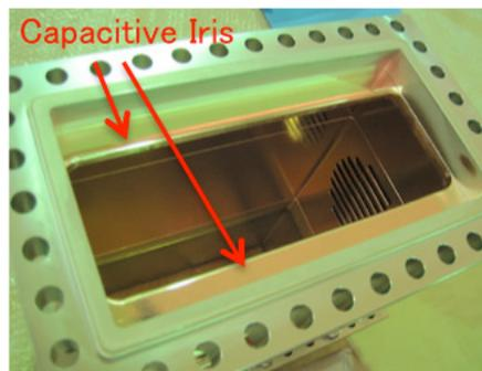
Figure 10: Manufactured waveguide which contains the capacitive iris.
