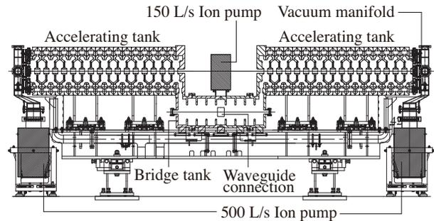
Figure 2: Accelerating cavity in the J-PARC ACS.
