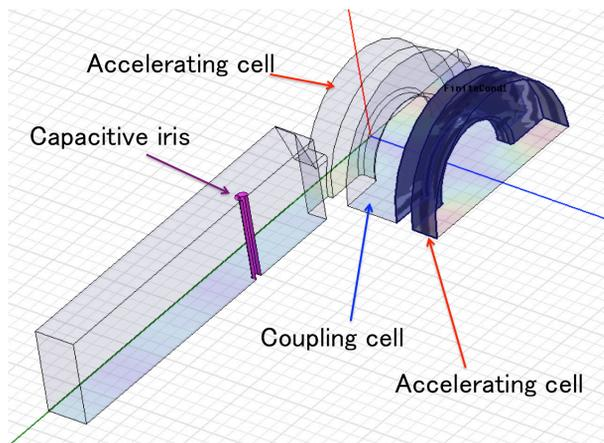
Figure 5: Analysis model for the bridge coupler.
