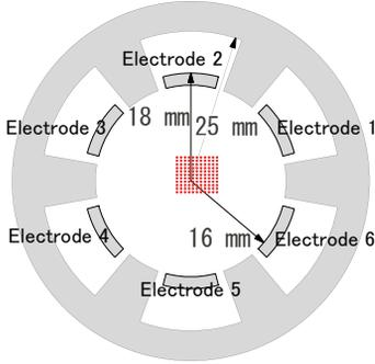
Figure 1: Cross-section of 6EBPM and mapping points (denoted by red circles) in entire calibration.
