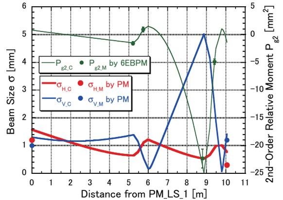
Figure 8: Calculated and measured  $\sigma_H$ ,  $\sigma_V$  and  $P_{g2}$ .
