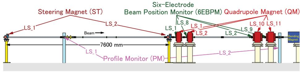
Figure 5: Schematic layout of equipment for emittance measurement.
