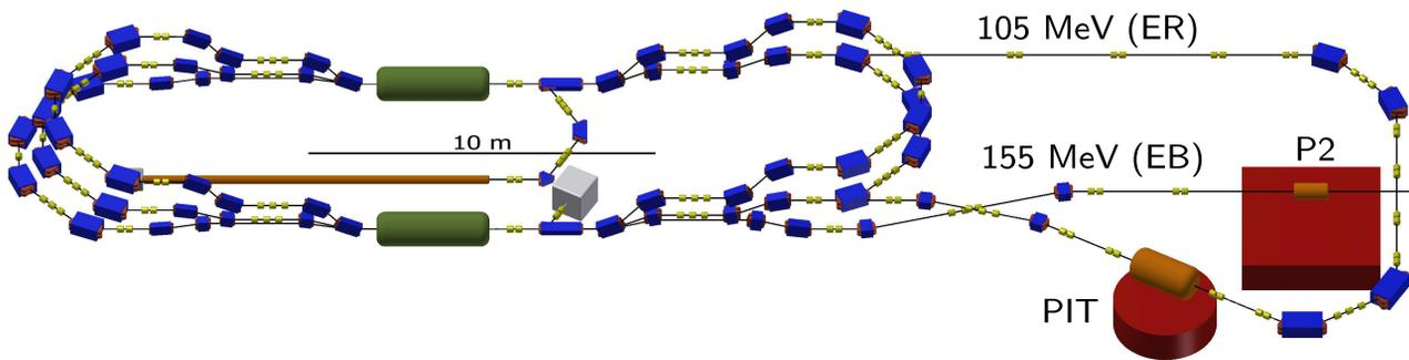
Figure 2: A 3D sketch of MESA: The main accelerator consists of two superconducting linac modules, the vertical beam separations and five 180° arcs. The experiments are an internal experiment for the ER mode with a beam energy of 105 MeV and an external experiment at 155 MeV. The red blocks mark the footprint area reserved for the experiments.
