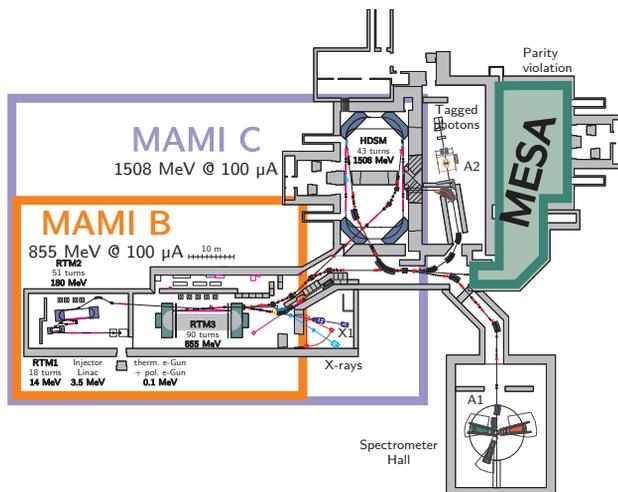
Figure 1: Floor plan of the MAMI accelerator. The space for MESA is marked in green.
