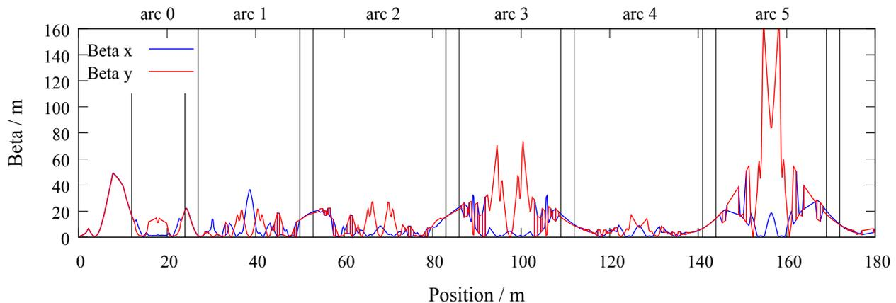
Figure 3: Beam beta functions of MESA in EB mode including space charge calculated with PARMELA.
