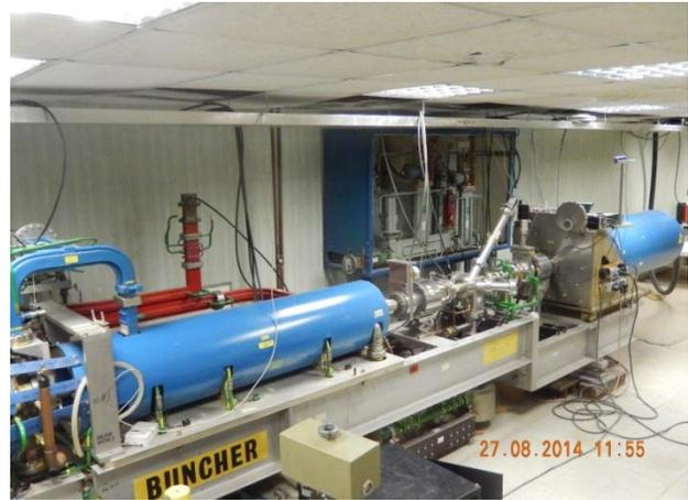
Figure 1: The electron injector.
