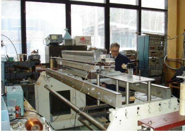
Figure 4: Configuring the undulator.
