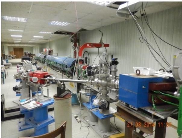
Figure 5: The bending magnet, undulator, drift gap and the accelerating section of the second accelerator station.
