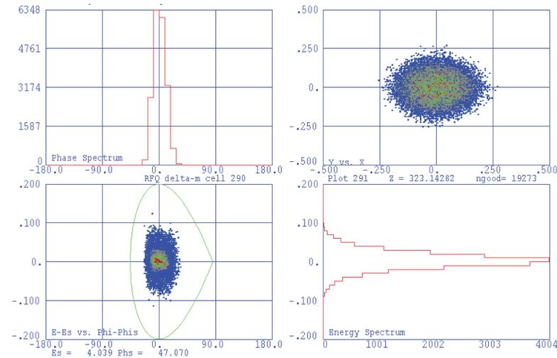
Figure 3: Output beam properties (upper left: phase spectrum, upper right: x vs y lower left:  $\Delta\phi$  vs  $\Delta E$ , lower right: energy spectrum)
