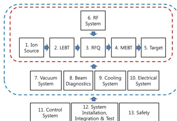
Figure 1: Block diagram of the helium irradiation system
