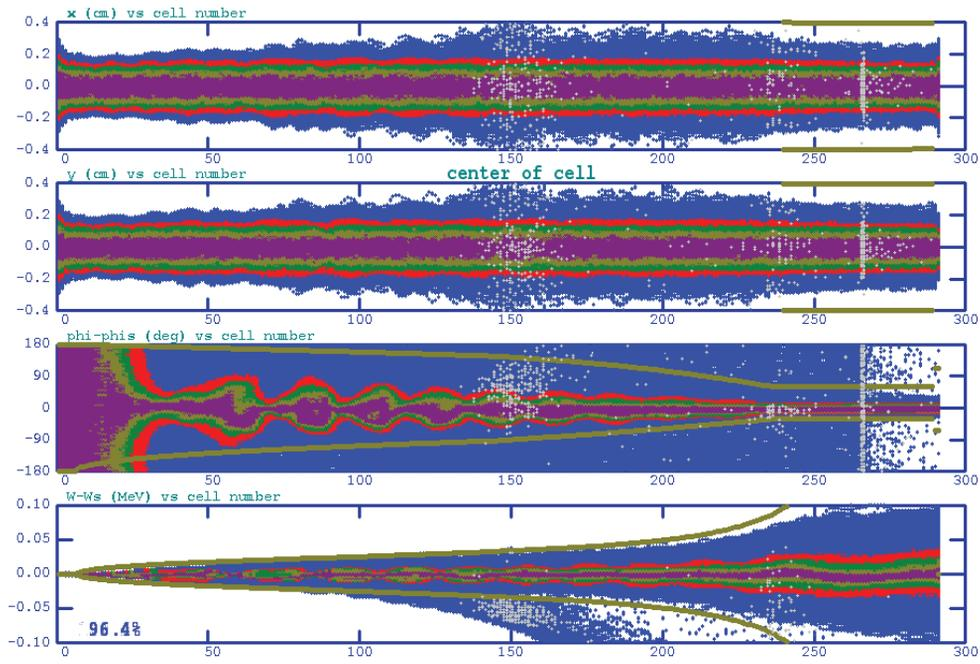
Figure 2: Beam trajectory through RFQ (1: x vs cell number, 2: y vs cell number, 3:  $\Delta\phi$  vs cell number, 4:  $\Delta E$  vs cell number)
