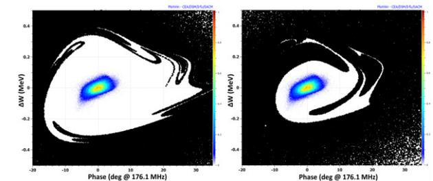
Figure 4: Longitudinal acceptance and input beam. Left: nominal tuning. Right: fault-recovery scenario.
