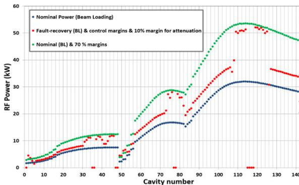
Figure 5: Estimation for the RF power requirements.
