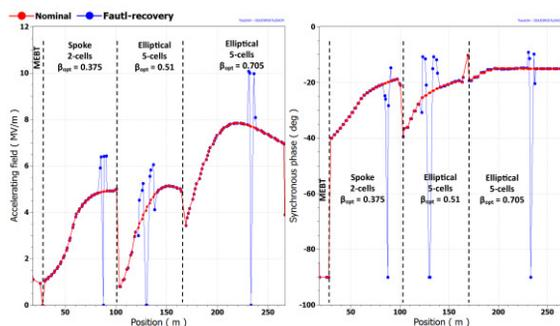
Figure 2: Example of multiple RF failures compensations with the local retuning method: accelerating fields (left) and synchronous phases (right).
