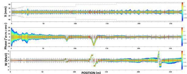
Figure 3: Beam dynamics with failures compensation.
