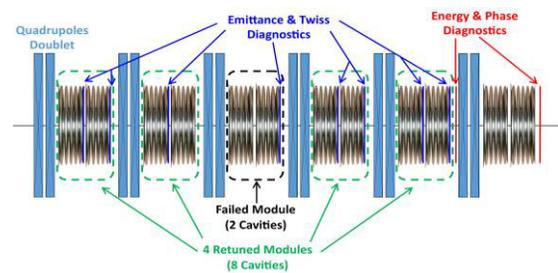
Figure 1: Principle of the local fault compensation method. Example of the retuning strategy used in TraceWin for the failure compensation of one cryomodule in the medium energy section ( $\beta_{\text{opt}}=0.51$ ).
