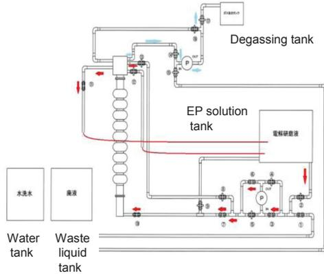
Figure 3: Schematic view of 9-cell cavity VEP facility.
