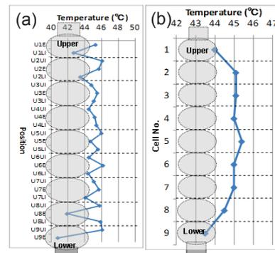
Figure 6: (a) Temperature of each part after 60 min VEP. (b) Temperature of the average of each cell after 60 min VEP.
