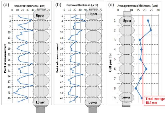
Figure 7: (a) Removal thickness of each part (one side along vertical direction). (b) Removal thickness of each part (180° opposite side of (a) along vertical direction). (c) Average removal thickness of each cell.
