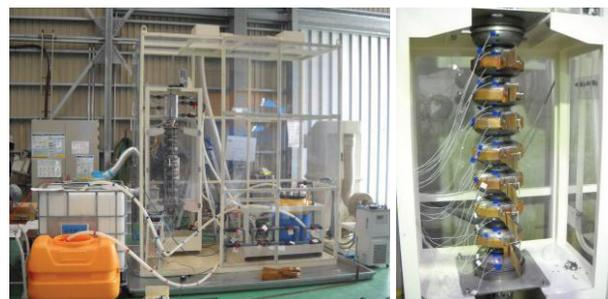
Figure 2: (Left) Picture of 9-cell cavity VEP facility. (Right) Picture of 9-cell cavity.
