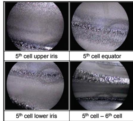
Figure 9: Images of inner surface of 5<sup>th</sup> cavity after VEP observed with an endoscope.
