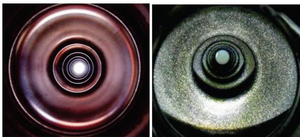
Figure 8: Images of inner surface observed with a digital camera. (Left) before VEP. (Right) after VEP.
