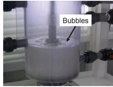
Figure 4: Picture of bubbles at upper side during VEP.
