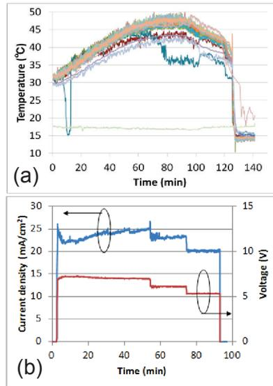
Figure 5: (a) Logged data of temperature of cavity during VEP. The detail of measurement position is omitted in this graph. (b) Logged data of current density and voltage during VEP.
