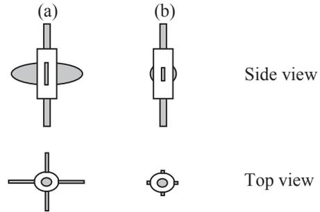
Figure 1: Schematic view of “i-cathode Ninja”<sup>®</sup>. (a) unfolded status. (b) retracted/folded status.
