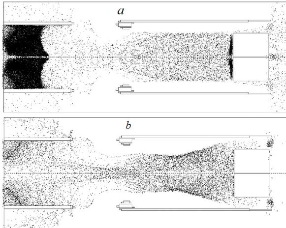
Figure 9: Electrons distributions for current 150mA (a) and 150 $\mu$ A (b).
