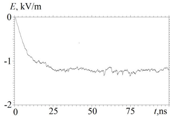
Figure 4: Longitudinal electric self-field time dependence near the cathode.
