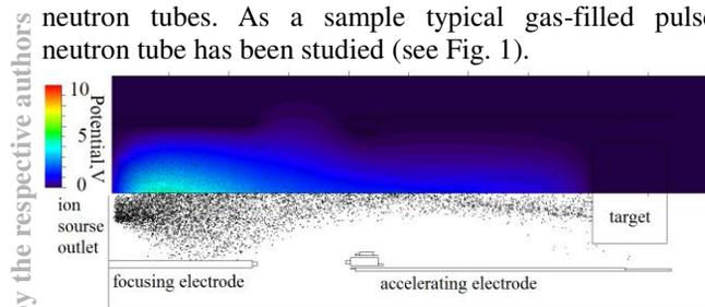
Figure 1: Deuterons distribution (lower) and their self-field potential (upper) in neutron tube.
