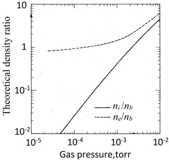
Figure 3: Ratio of electron or ion density as a function of pressure.
