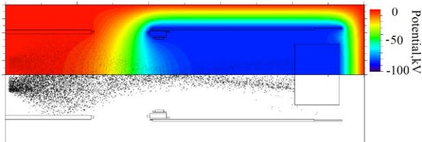
Figure 5: Deuterons distribution (lower) and total field (external and self-field) potential (upper) in neutron tube.
