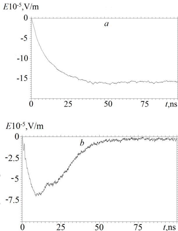
Figure 10: Longitudinal electric field time dependence without (a) and with (b) ionization taking into account.
