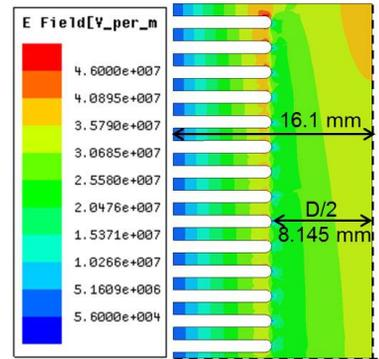
Figure 5: Electric field distribution for 300 MW input power over one quarter of the H-plane of the constant impedance section.
