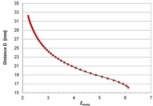
Figure 6: The distance  $D$  versus the impedance  $Z$  along the matching taper.
