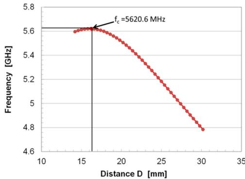
Figure 4: Cut-off frequency varying the distance  $D$  between two opposite ridges.
