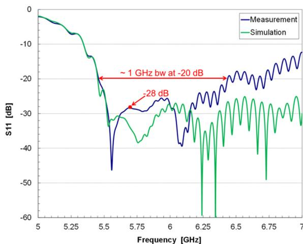
Figure 8: S11 frequency spectrum from cold measurement (blue line) e from analytical computation (green line).
