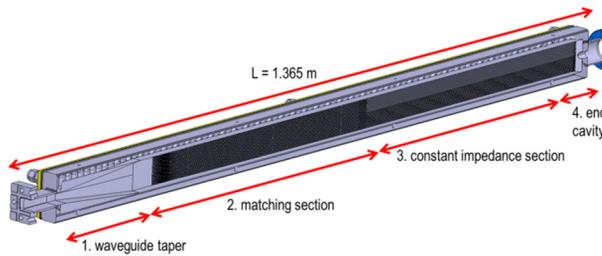
Figure 3: The four waveguide sections which compose the C-band high-power load.
