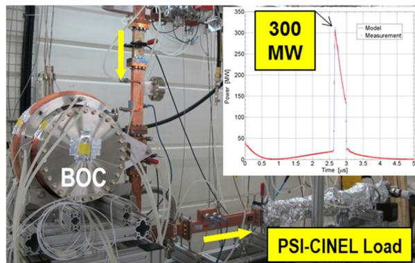
Figure 9: High-power test of the BOC prototype. The dry load absorbs up to 300 MW peak power produced by the pulse compressor in phase jump operation. In the plot the compressed pulse of the BOC.
