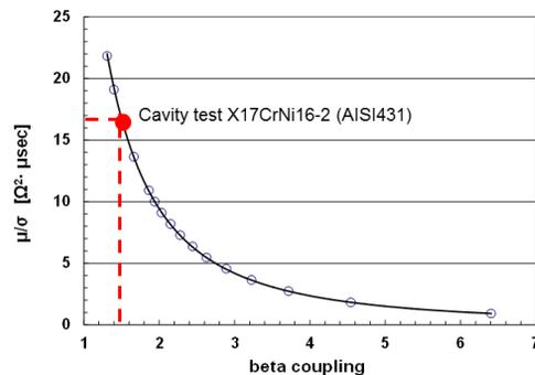
Figure 2: Simulated curve of the ratio  $\mu/\sigma$  versus the  $\beta$  coupling. The red circle represents one of the tested material, the magnetic steel AISI431.
