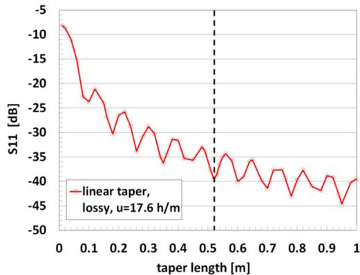
Figure 7: The taper reflection S11 for different lengths.
