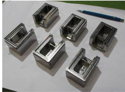
Figure 1: Sections of the cavity test used to determine the best magnetic steel for the load.
