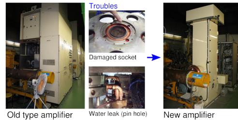
Figure 2: Old power amplifier, its troubles, and a new amplifier constructed in FY2013.
