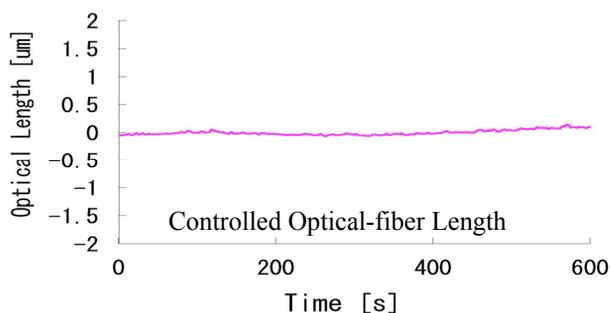
Figure 7: Control performance of the optical-fiber length control system. The fiber length is regulated within  $1\ \mu\text{m}$  in the case of only the fine control.
