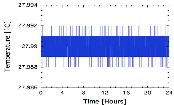
Figure 5: Temperature control performance of the 238 MHz sub-harmonic buncher. The temperature is regulated within  $\pm 2 \text{ mK}$  (p-p).
