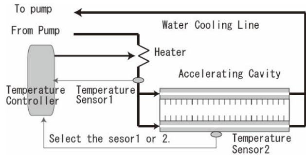
Figure 4: Highly precision cavity temperature controller.
