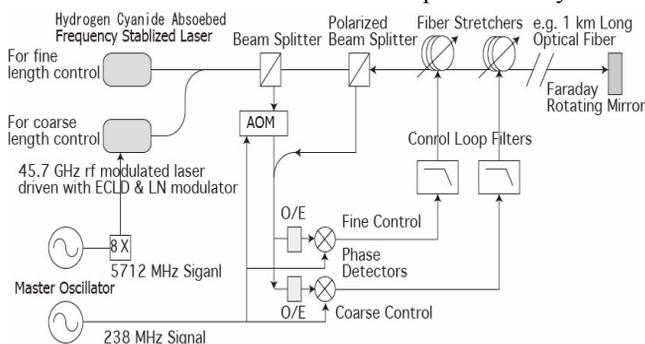
Figure 6: Optical-fiber length control system.
