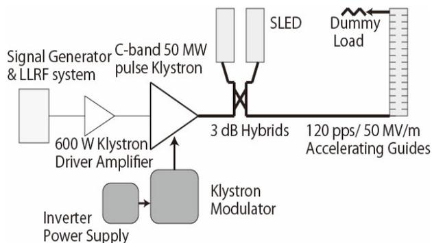
Figure 1: Experimental set-up of the 120 pps C-band acceleration unit.
