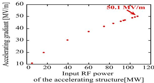
Figure 3: Acceleration gradients of the  $2\pi/3$  CG accelerating structure, as a function of its input rf powers. These gradients are calculated by using a shunt impedance of  $64 \text{ M}\Omega/\text{m}$ .
