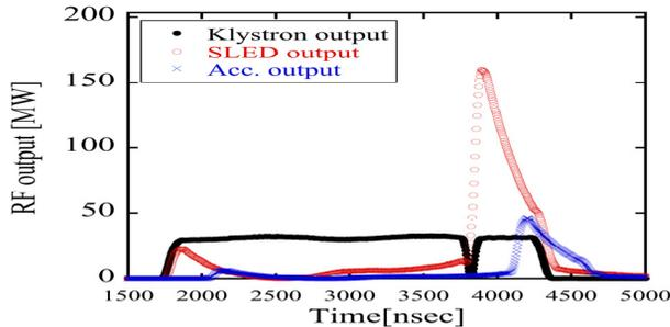
Figure 2: Rf power wave forms at 120 pps.
